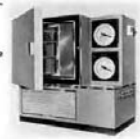
Low temperature & humidity chamber "Lucifer" (1961)
