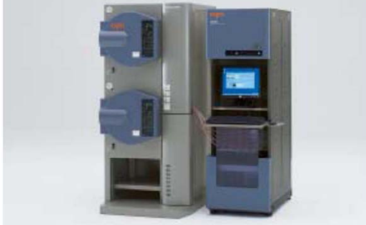
Example of the Highly accelerated stress test system with the Ion migration evaluation system
